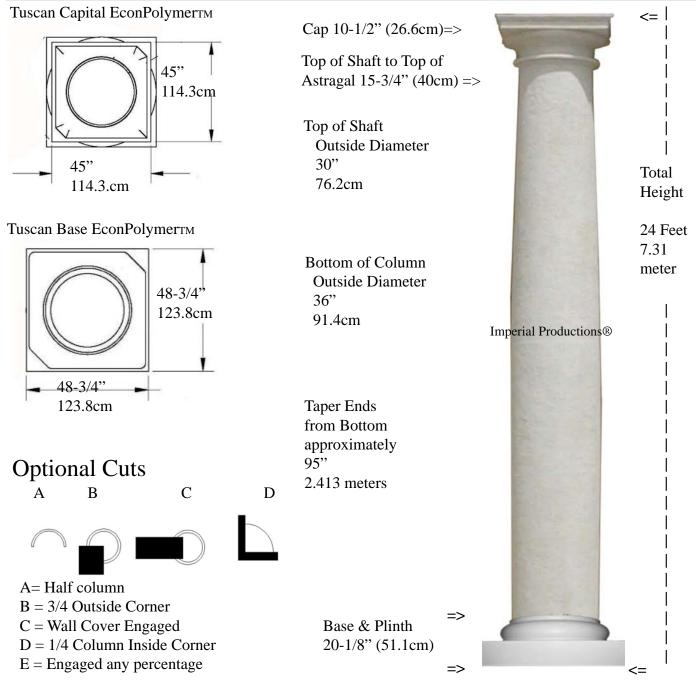
Weight Shaft 887 lb (402.34 Kg) Centered Load to 20,000lbs (9.07m tons)
