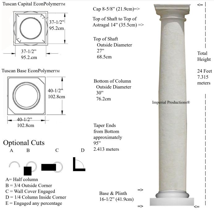
Weight Shaft 709 lb (321.6 Kg) Centered Load to 20,000lbs (9.07m tons)
