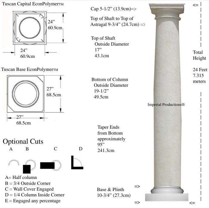
Weight Shaft 428 lb (194.14 Kg) Centered Load to 20,000lbs (9.07m tons)
