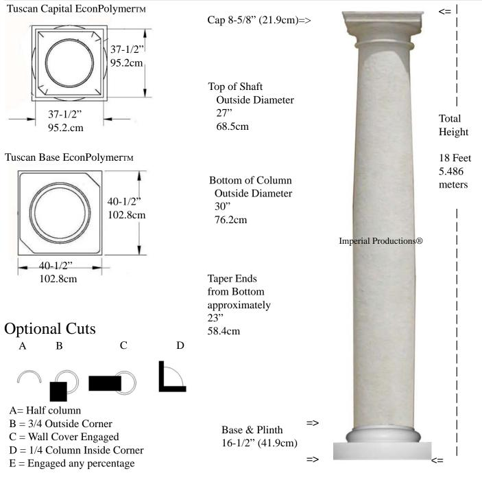
Weight Shaft 528lb (239.5Kg) Centered Load to 20,000lbs (9.07m tons)
