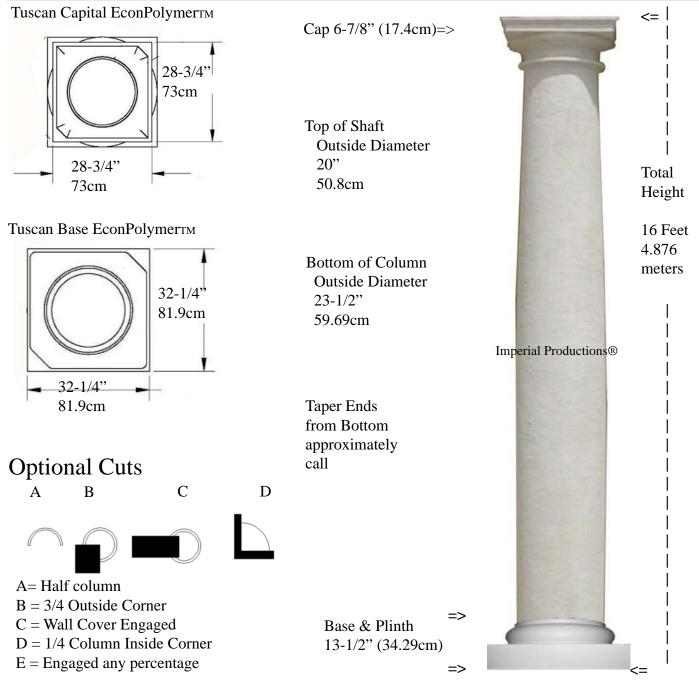
Weight Shaft 328 lb (148.8 Kg) Centered Load to 20,000lbs (9.07m tons)
