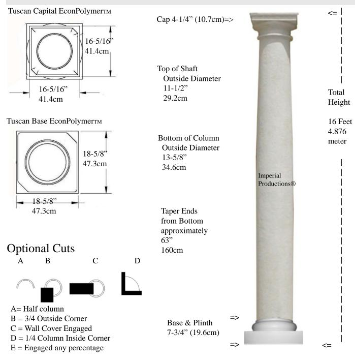
Weight Shaft 226 lb (102.5 Kg) Centered Load to 20,000lbs (9.07m tons)
