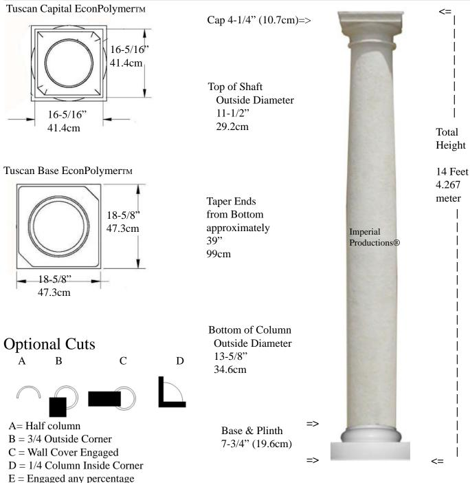
Weight Shaft 199 lb (90.26 Kg) Centered Load to 20,000lbs (9.07m tons)
