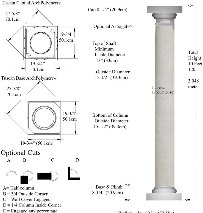
Shaft weight 160 lbs (72.5kg) Center Loads to 20,000lbs (9.07m tons)
