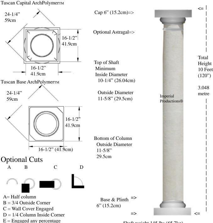
Shaft weight 145 lbs (65.7kg) Center Loads to 18,000lbs (8.164m tons)
